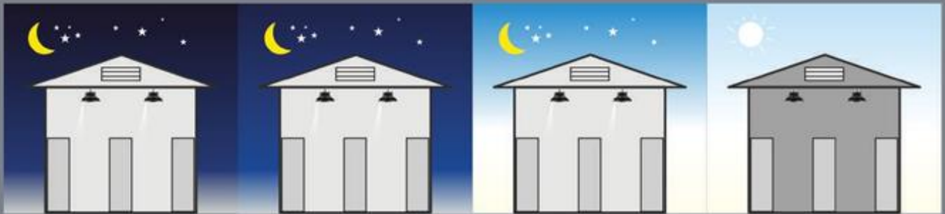
Keep actual illuminance (natural light+lamp light) at a setting value in a workplace.
