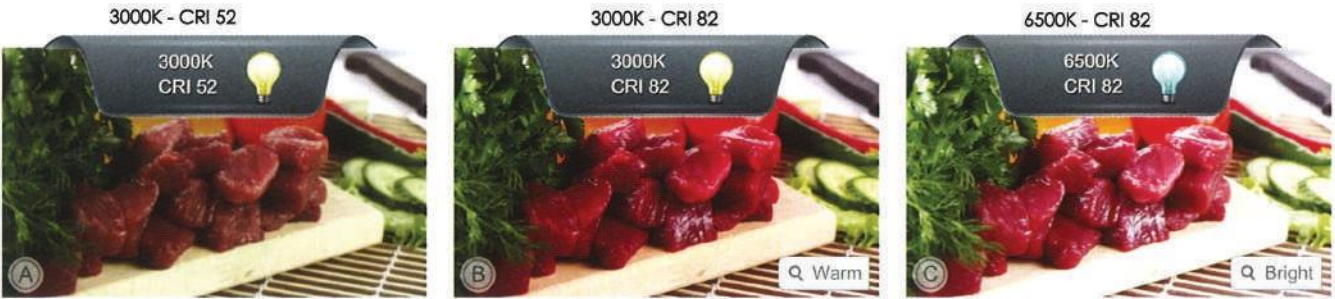
A and B light : The color of the object looks better when under B light.
