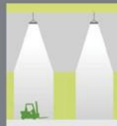
Lamps will automatically shut down when ambient illuminance reaches setting value.
